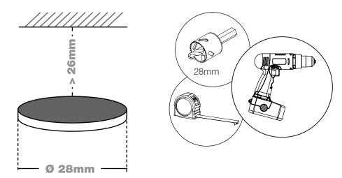
To install the LED recessed spotlights in walls, ceilings or in the inner rafters of patio roofs (see page 6), Ø28 mm holes must be drilled at the desired positions, through which the connecting cable must also be routed.
